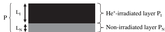
Fig. 6. Simple resistance model of gas permeability through the two-layer surfaces in ion-irradiated asymmetric polyimide membrane.
